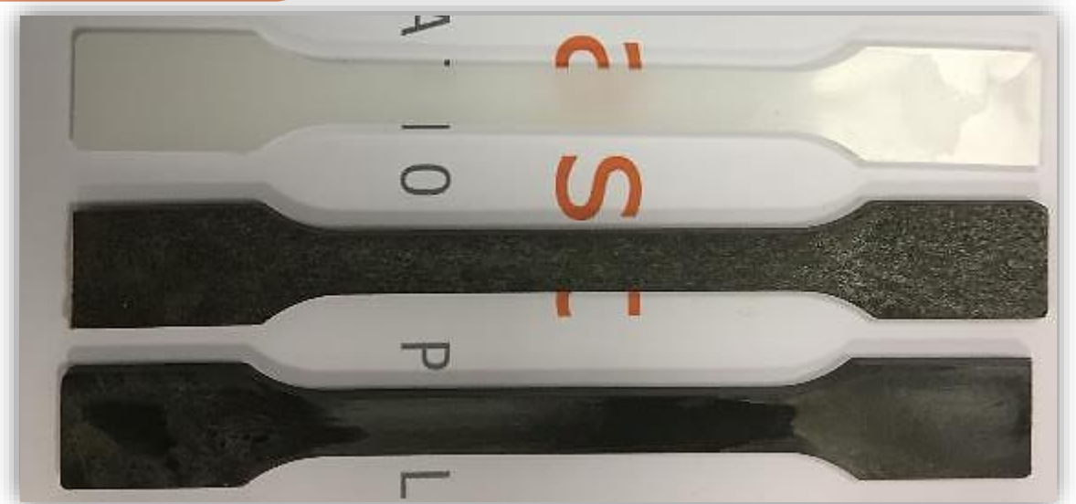
Injection moulding of specimens for characterization tests
